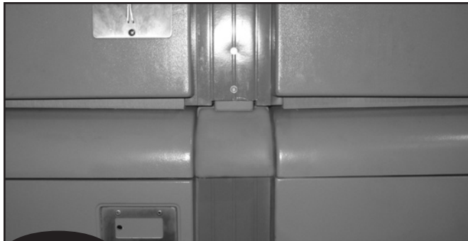
FIG. 4 Center Support Block properly aligned.
